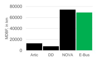
Figure 3: Propulsion MDBF Comparison, in km
