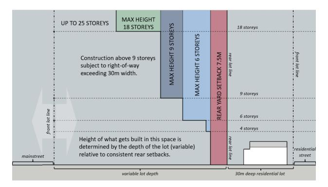
Profile of a site showing fixed setbacks and height graduations relative to a variable lot depth; built form will vary with lot depth.
